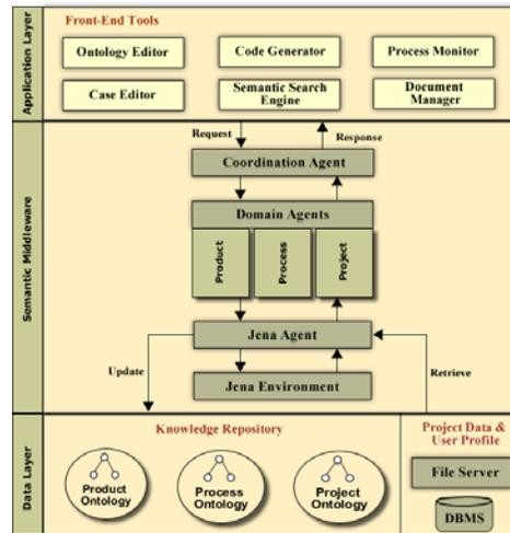
**Figure- 1.** Tool Architecture
